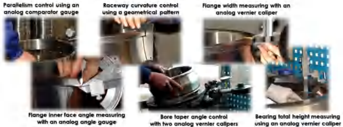
Fig. 19 – Measurements within integral calibrated system
