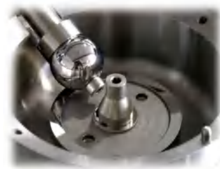
Fig. 6 – Ball-on-washer life prediction testing rig
