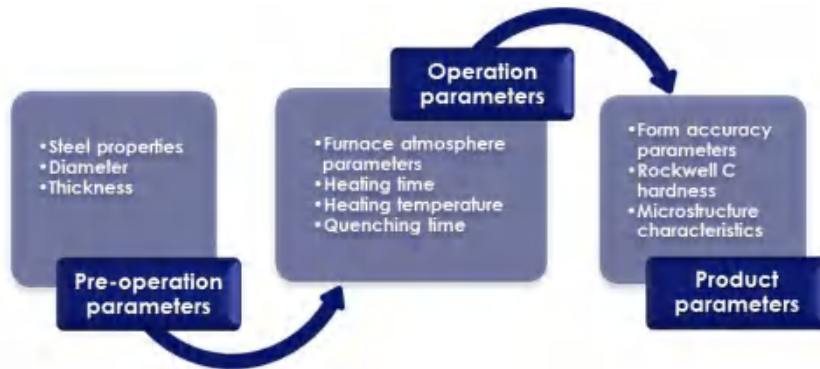
Fig. 16 – Heat treatment quality parameters
