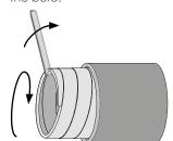
Note: Do not axially screw the spiral outer ring by means of locknut or similar tools!
