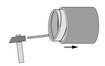
Should you install wound bearings featuring a bore diameter larger than 250 mm, BUT suggests to use proper tapered rings to easy the mounting. In fact these tapered rings facilitate the insertion of the cage with rolling elements onto the spring rings.
